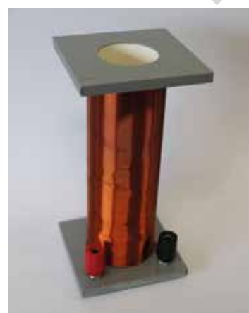
FIGURE 3 An air-cored solenoid of 200 turns
