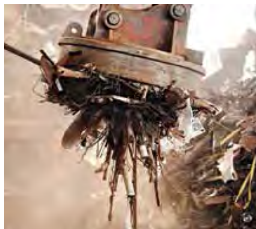
Figure 2.12 Magnets are used to separate metals in recycling plants.
