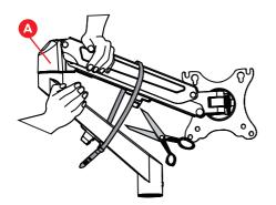
Firmly hold the 2 halves of the spring arm together and have another person cut off the cable tie from around the spring arm.
